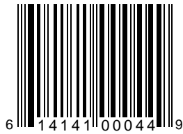
UPC-A symbol GTIN-12 structure
